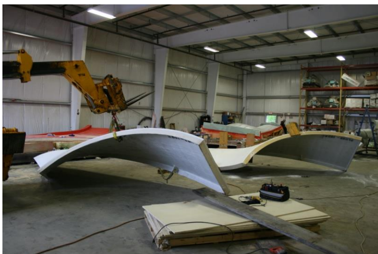
Composite "Blubs" out of their mold
